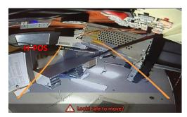
In H-POSITION, use  $\triangleleft$ ,  $\triangleright$  on remote control, to adjust parking guideline left and right.
