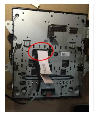
② Take out cables through the marked place and assemble the plate.
