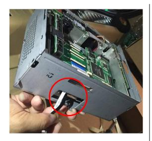
Pull the cables on the backside of LCD through the marked place.
