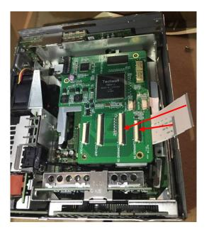
⑥ On the top of bracket, place the subboard and connect the supplied FFC cables as shown on the left
