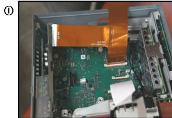
LVDS FPC cable connection
