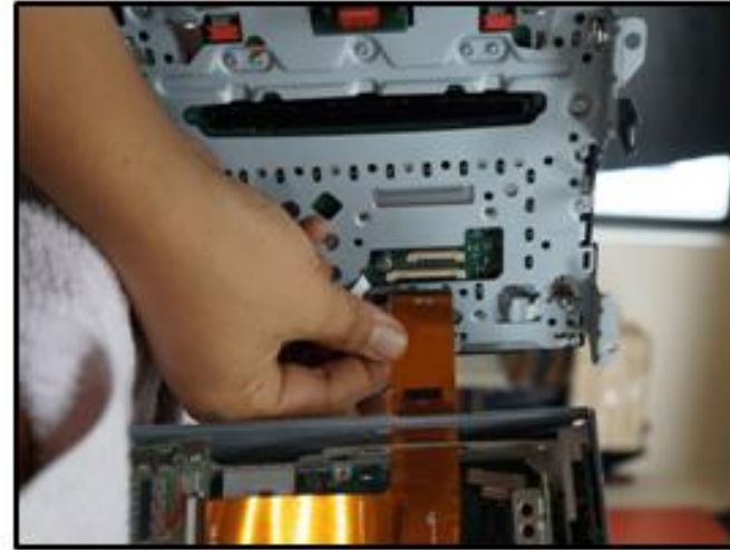
LVDS FPC cable connection
