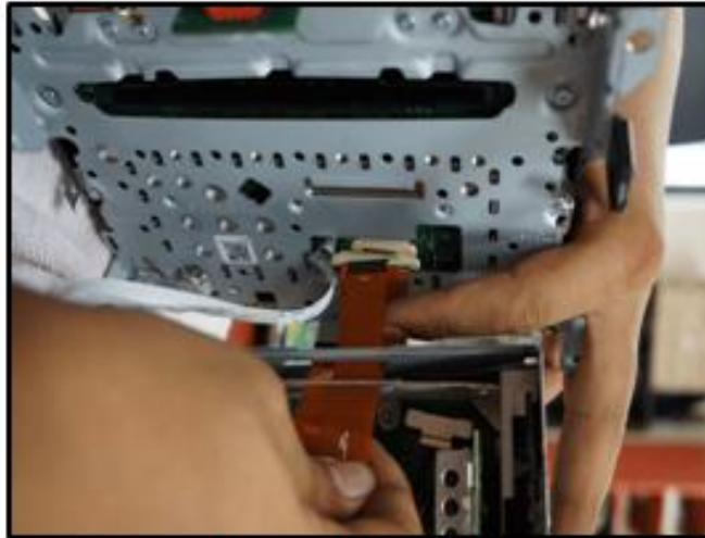
Key FPC cable connection
