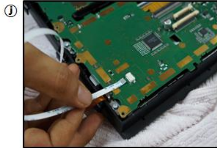
Touch OUT cable connection
