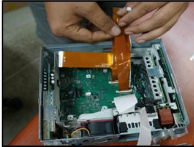
Key FPC cable connection
