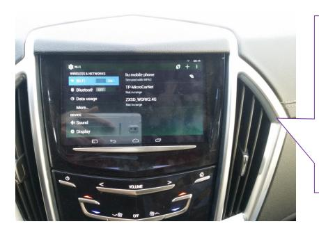
Enable the wifi, in order to get the Traffic situation when driving, the driver should enable his phone's hot-spot. Thus the navigation software inside this module can get internet from 3G/4G mobile network.
