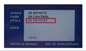
Press ◀ button or UP→DOWN→UP→MENU button of remote to run factory menu and then choose UTIL2→ IR MEMORY→NAVI
