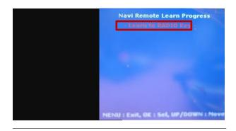
2 After Step1. you will see image like above picture. System shows each MMI button name for your navigation button matching. Just press okay, if this is not the button you want, press up, down buttons to change to other MMI button.
