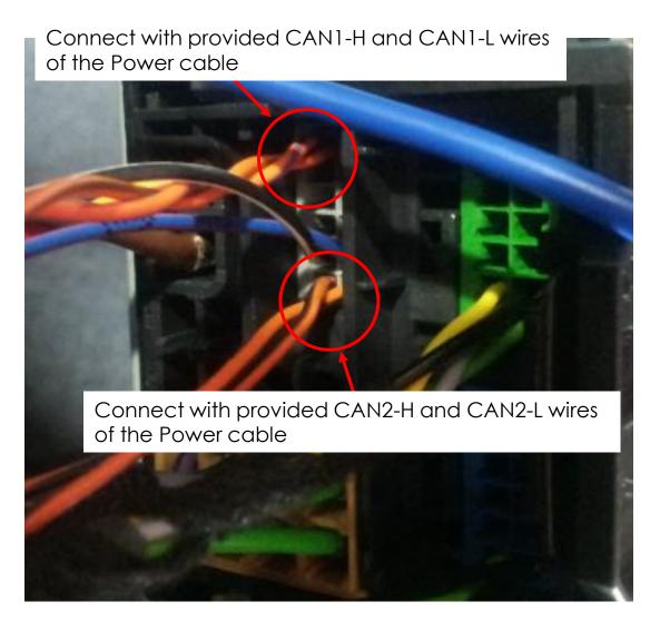
In case of some problem comes up if connect the wires, Try to change the CAN1 and CAN2
