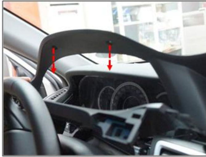
Pull out the Bolts
