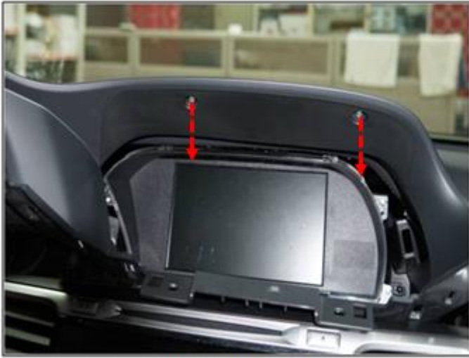
Pull out the Bolts
