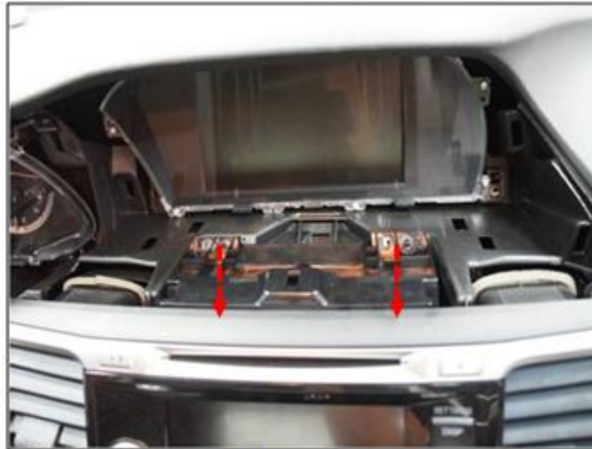
Pull out the Bolts
