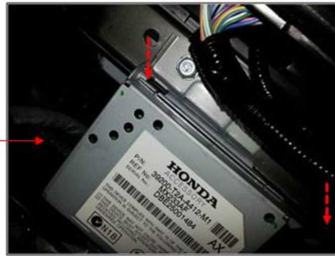
Pull out the Bolts
