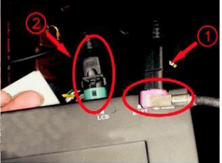
5. Position 1 in pic. should be connected to Position 2 (LVDS video input of Interface).
