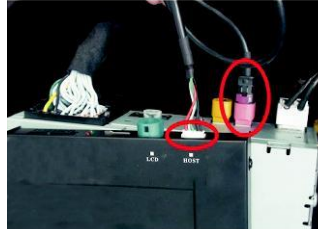
6. Connect LVDS video cable of interface to car original LVDS position at the rear of main unit.
