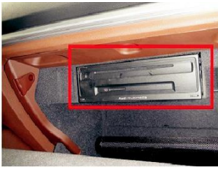
1. Open car glove-box, and take out of inside main unit with special removal kits.
